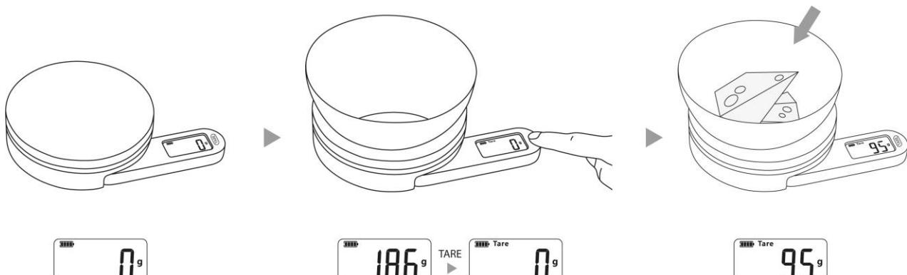
Place an empty container on the scale. The display will now show the weight of the container. Touch the TARE button and the display shows zero "0" and clears the weight of container.
