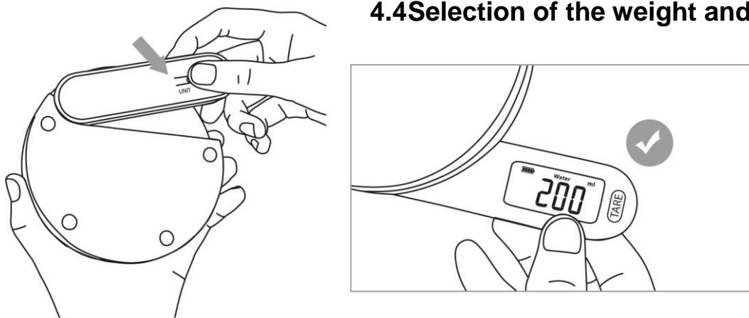
Press the UNIT button (at backside of display) to interchange the unit between g, oz, Water ml, Milk ml. Select the UNIT button before weighing. The TARE button cannot be pressed at the same time as the UNIT button.
