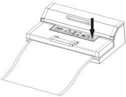
Press “Manuelles Schweißen” (manual seal) button to start sealing the bags. The status Indicator D light. Once it is finished, light will turn off.
