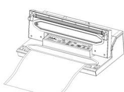
Put one end of the bag on top of the sealing strip, but not enter the vacuum chamber.
