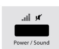
Press the button **power/sound** for three seconds in order to switch on or off the sound (beep tone).
