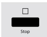
To terminate the interrupted program, press the button **Stop** a second time.
