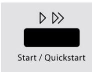
After selecting the temperature, press the button **Start /Quick start**. A signal ton is emitted and the **PREH** display blinks until the oven has reached the programmed temperature.
