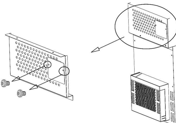
Carefully loosen the screws.
