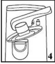
To release, grasp the can firmly in one hand and raise the lever using the other hand. The magnetic lid lifter will retain the lid as shown in figure 4.
